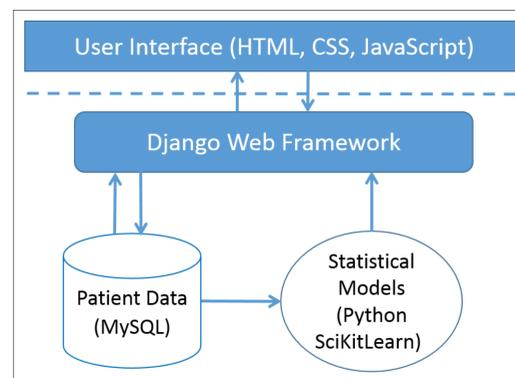
**Figure 2.** Components of the LEMUR system.
